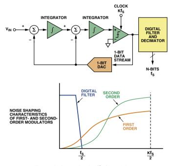
Figure 8. Second-order  $\Sigma$ - $\Delta$  modulator.
