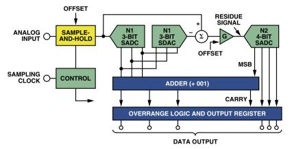
Figure 14. 6-bit subranging error-corrected ADC, N1 = 3, N2 = 4.
