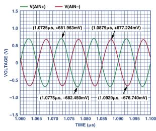
Figure 3a. 100-MHz input. Simulation of the transformer's secondary outputs: AIN+ (green) = 1.364 V p-p, AIN- (red) = 1.354 V p-p, Difference = 10.45 mV p-p.
