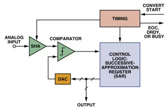
Figure 2. Basic successive-approximation (SAR) ADC.
