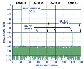
Figure 5. 4-channel time-interleaving FFT.
