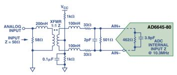
Figure 10. Switched-capacitor front-end implementation.
