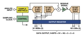
Figure 11. 6-bit, two-stage subranging ADC.
