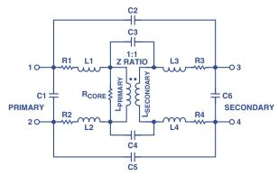
Figure 1b. Typical transformer model.
