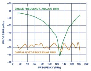
Figure 6. AD12400 wide-band image-spur performance.
