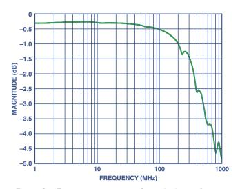
Figure 8a. Frequency response of a typical transformer.
