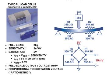
Figure 9. Load-cell signal-conditioning application.
