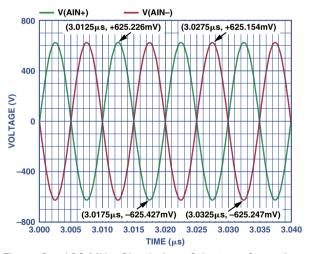
Figure 6a. 100 MHz. Simulation of the transformer's secondary outputs: AIN+ (green) = 1.25 V p-p, AIN-(red) = 1.25 V p-p, Difference = 0.25 mV p-p.
