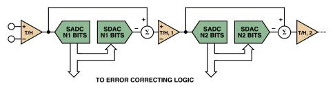
Figure 15. Generalized pipeline stages in a subranging ADC with error correction.
