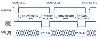
Figure 3. Simplified timing diagram of a SAR A/D converter.
