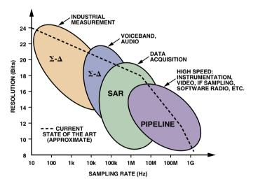
Figure 1. ADC architectures, applications, resolution, and sampling rates.
