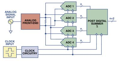
Figure 1. Summing four ADCs in parallel.
