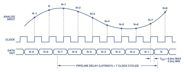
Figure 16. Timing of a typical pipelined ADC, the 12-bit, 65-MSPS AD9235.
