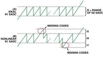
Figure 12. Residue waveform at input of second-stage SADC.
