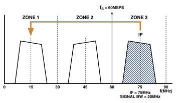
Figure 18. Sampling a 20-MHz BW signal with an IF frequency of 75 MHz at a sampling rate of 60 MSPS.
