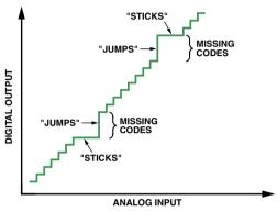
Figure 13. Missing codes due to MSB ADC nonlinearity or interstage misalignment.
